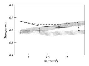
FIG. 1. Nuclear transparency extracted from  ${}^4\text{He}(\gamma, p\pi^-)$  vs squared momentum transfer |t| at  $\theta_{\text{c.m.}}^\pi = 70^\circ$ . Solid (dashed) curve is the result of the RMSGA calculations without (with) color transparency. Semiclassical model [16] results are presented by the shaded areas: hatched (dotted) area is a calculation without (with) CT. Data from Ref. [14].
